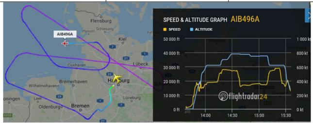
.. since with the change of track direction the ground speed varies considerably, pointing to high winds. The sequence of altitude steps can be interpreted as a condensed test pattern. The descend to an altitude near FL100 over the North Sea is unusual. The observation was abandoned due to organizational reasons and could not be picked up in time.
